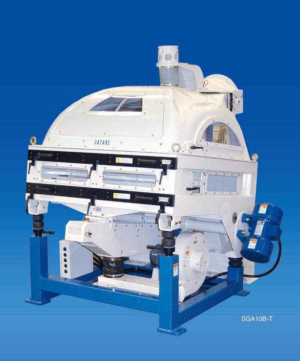
The Satake Destoner SGA concentrates impurities for more efficient separation by subsequent machines.
